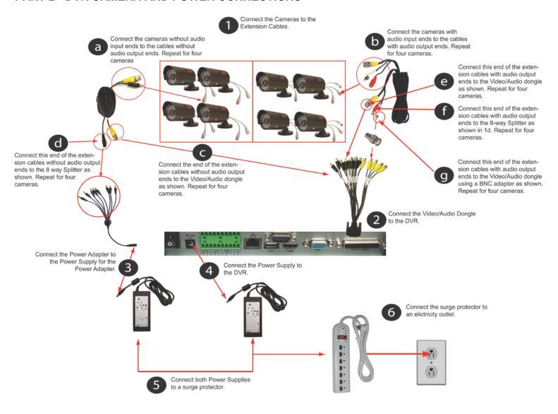
Please note that it is STRONGLY recommended to use a surge protector that is UL-1449 rated. Look for a clamping voltage of 330 or lower, a Joule rating of at least 400 and a response time of 10 nanoseconds or less.
